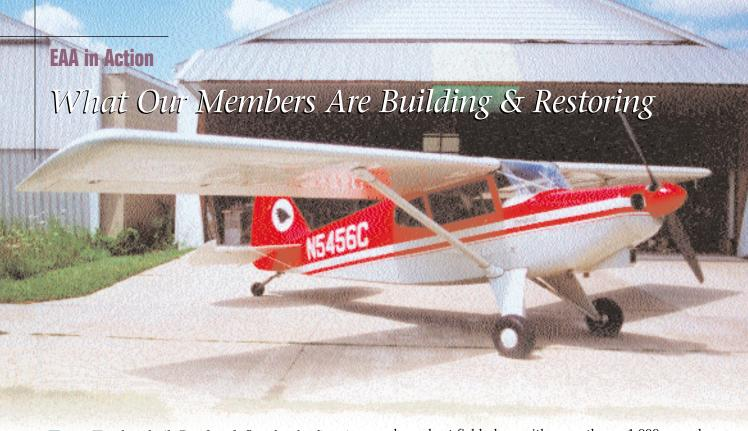
y plans-built **Bearhawk** flew for the first time on July 6, 2001, after two-and-a-half years of construction. At the time of the first flight, the plane was missing the electrical system, avionics, and many refinements. It took another year to complete and finish as an IFR platform. It cruises at 150 mph (75 percent power) with the 230-hp O-470 and a Hartzell constant-speed propeller. It's a great four-
