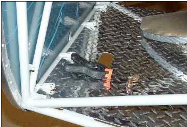
Diamond plate aluminum isn't going to be the lightest floor boards, but this builder was looking for rugged durability. We'd say he got it.
