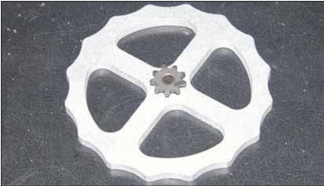
The trim wheel from AviPro clears the fabric. It is designed for 1/4" roller chain available at hardware stores. Attach the 1/16" cable by threading it through the end links and nicopressing.
