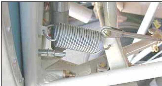
This is the correct rudder return spring and will do a much better job than the smaller ones.
