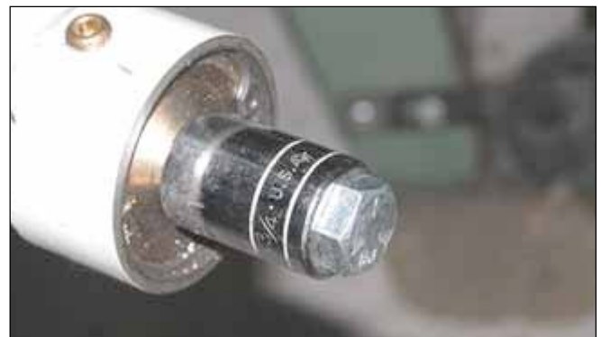
When installing the internals in the strut, it is much easier if you compress the spring using the above method--run a bolt through a socket and compress just enough to get the snap ring in the groove.
