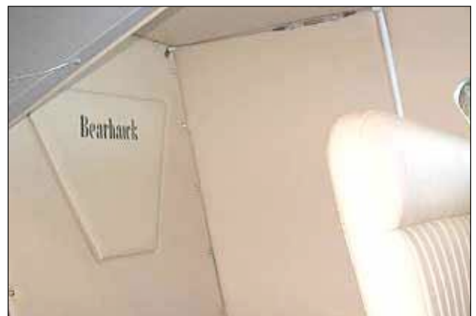
This trapezoidal opening is the maximum size possible and parallels the tubing behind it. This one is hinged upward for easy access to cables, etc.
