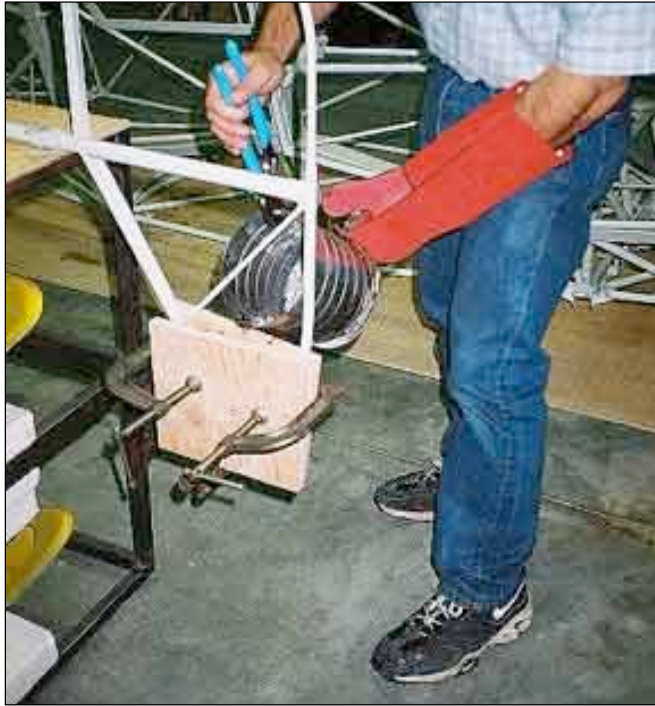
Pouring lead. Note form is just 1/4" plywood clamed tight to tail. Drill holes in tabs and put screws in edge of tubing before pouring. to give lead attach points USE A FACE MASK, RESPERATOR AND DO IT OUTSIDE OR WITH PLENTY OF VENTLATION. LEAD IS NASTY STUFF!
