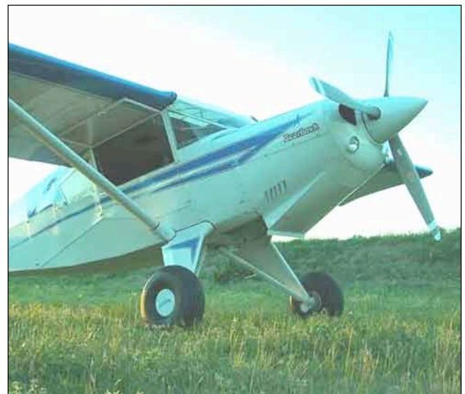
Robbie Staton hung a three-blade on the front of his fire breathing, Monte Barrett, cold air induction 540 hotrod.
