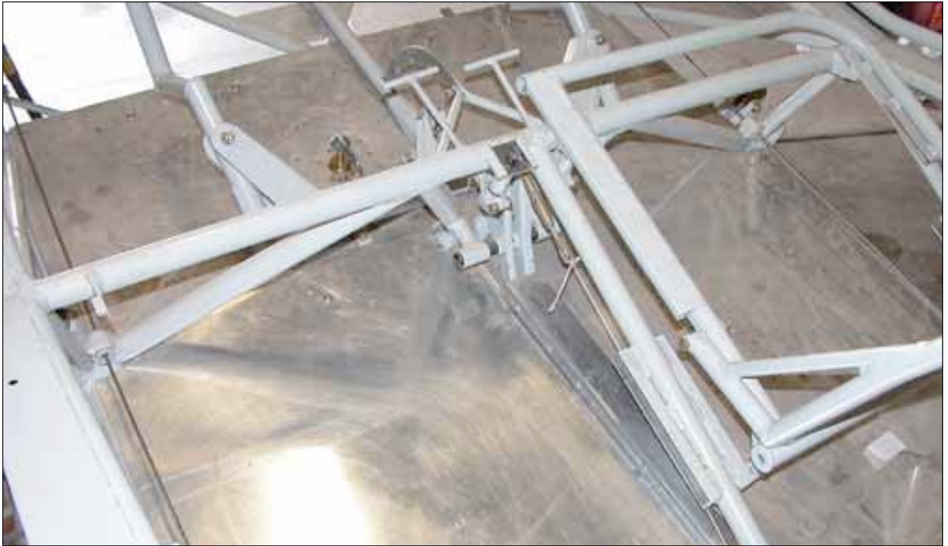
View from rear: The rear floor boards are often done in different ways. Here they are done in an elegant, simple manner: they are two panels, one each side with a vertical lip down each side. Notice in the middle where the vertical lips are joined with a simple cover that lets the flap cable come down through the rear of it. The center flanges add significant stiffness to the floor. It's worth noting that they were designed and fabricated by Phoenix builder Scott Williamson's wife, May Beth.
