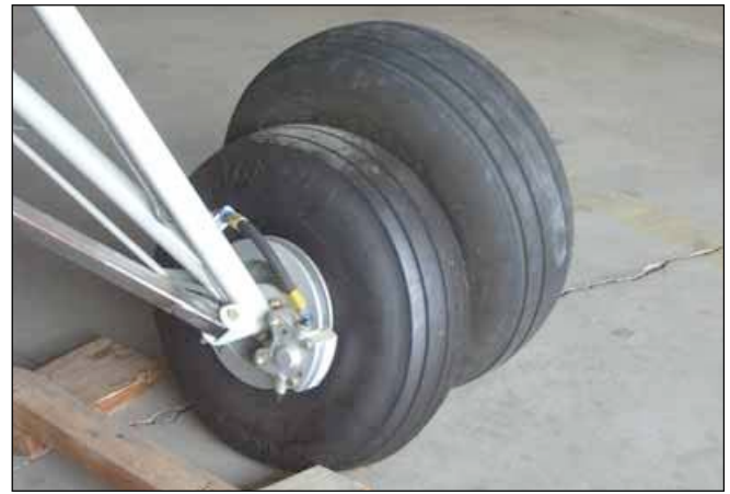
The 600 x 6 tire will handle 99% of most Bearhawkers flying, but many go for the 7.00, as shown here, "just in case." The 8.50 is significantly larger and heavier and slows the airplane quite a bit.
