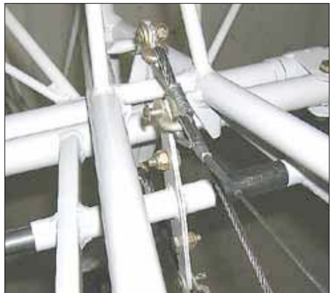
Another view showing how the trim and elevator cables are routed.
