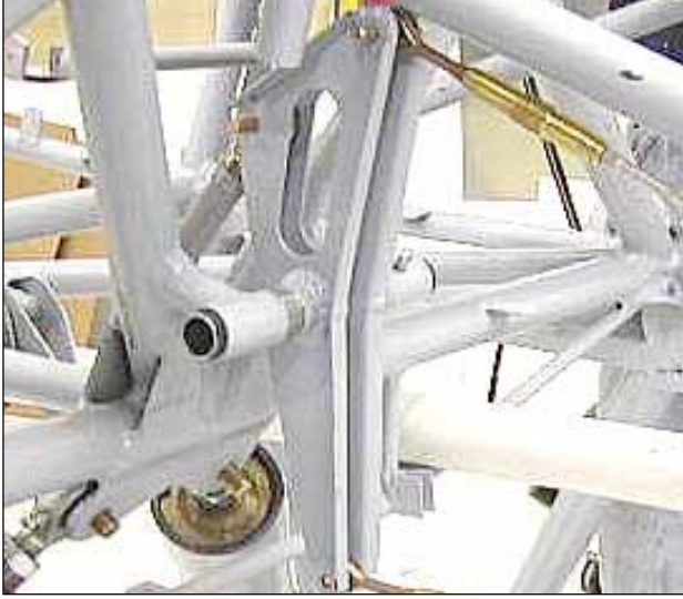
Elevator bellcrank as seen from left, rear: Use tubing spacers to move it slightly off center to avoid interference with flap cable. Cable from top of bellcrank goes to the left pulley behind it and bottom cable goes through the middle pulley.
