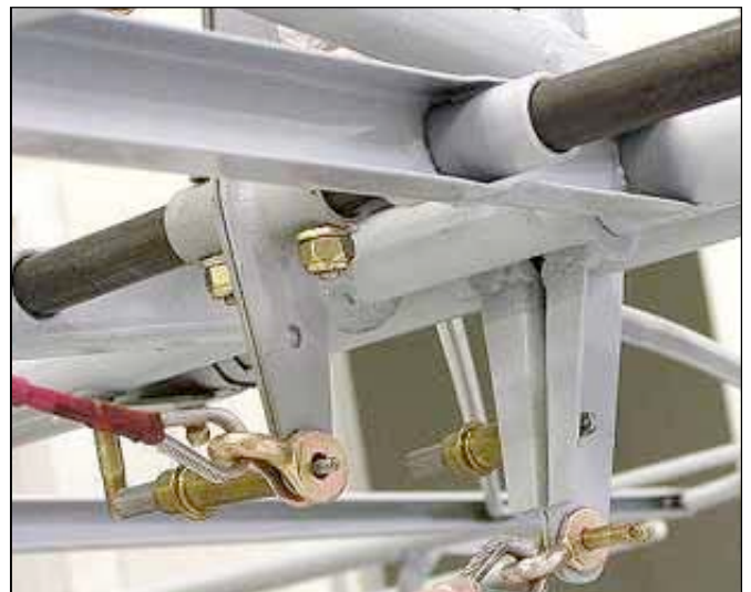
Install the black trim tab actuating tubes before assembling stab halves. Orient the bellcrank vertically and drill the holes, then do the same for the actuating arm on the outboard ends of the same tubes. Note the trim cable running from the bottom and top of the trim tab actuating arms. See trim wheel photo further on for more information.
