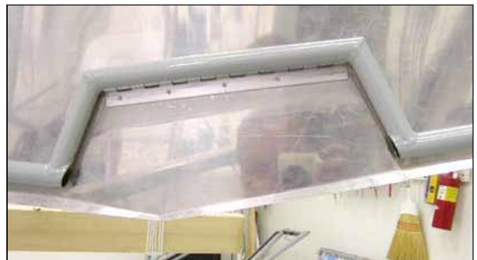
The famous Bearhawk "mouse door," which is necessary to allow the door to open wider. A simple piano hinge is attached and the mouse door skin is lapped to the inside of the main door skin, so that when the door is closed, the mousedoor is automatically sealed shut. Note that there is a slight break at the edges of the door skin to give a better seal.
