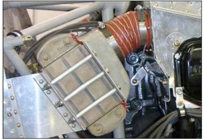
This is a good example of mounting the oil cooler, but efficiency would be improved with a longer plenum, which would give the air more time to slow down. See below picture.
