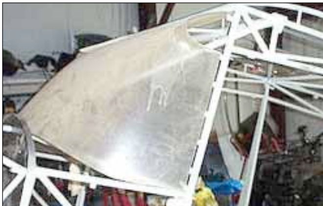
The windshield comes fairly well trimmed on the sides, but the top, where it goes into the channel, and the bottom, where it curves over the boot cowl, need to be trimmed.
