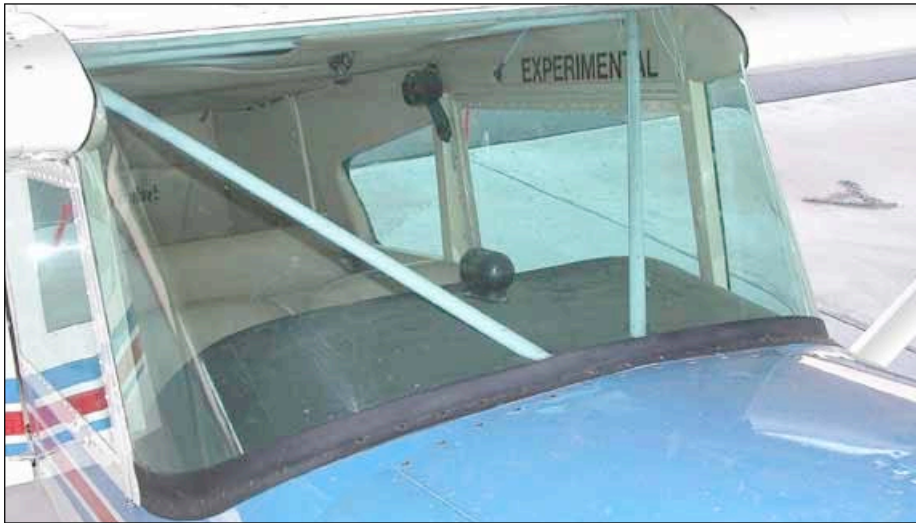
The windshield is available from L & P plastics trimmed close to net, but you'll still have to do some grinding. It's available in tints with gray being the most popular
