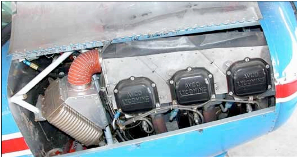
The engine cowling can't be accurately installed until the engine is hung and the spinner and prop are mounted because the nose bowl, and the entire cowling, indexes to the spinner.
