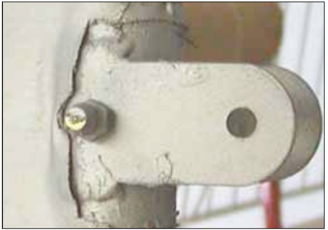
With this kind of elevator/rudder hinge, getting a neat, tight fit is a real challenge. some builders have fabricated "U" shaped pieces to go under the fabric to give the fabric something to glue to right at the cut edge shown here which cleans up the appearance considerably.
