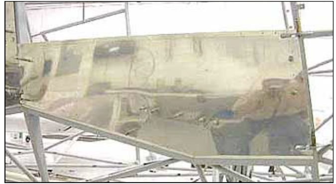
PK screws or pop rivets can be used to attach the skin, but using countersunk fasteners give a cleaner look.
