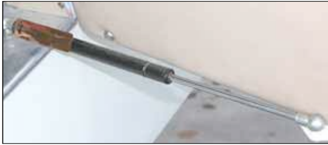
Rear door gas strut hold open device: this is so slick you shouldn't build the airplane without it. "Door Steward", WWW.mtnviewaviation.com , PN200C101. An automotive unit will be much less expensive, see www.allegiscorp.com
