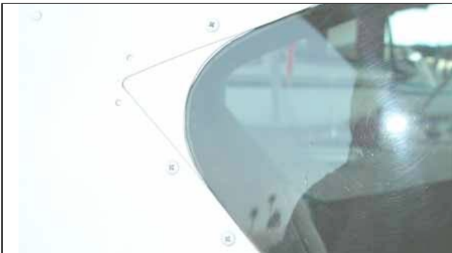
Some builders round the rear window corners w/filler pieces..
