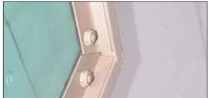
The .025 L-shaped strips hold the plexi against the door skin.
