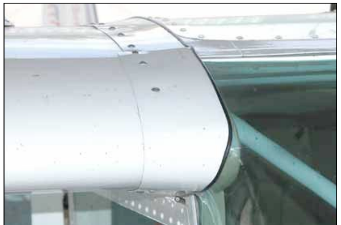
You want to get the windshield relationship to the wing just right to make your fairings fit better.
