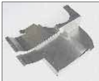
Van's Aircraft makes a complete baffle set for their RV-10 that is an excellent start for 540 Bearhawks.
