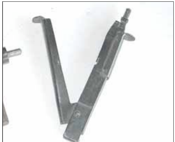
The hand nibbler is a simple tool that will let you cut square holes and edges in aluminum with ease and virtually no distortion.
