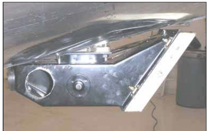
Sideview of lower cowl before the scoop is attached: Each installation will be slightly different but the air box will protrude and should be in place before the airscoop is positioned. Also, the hole shown where the alternate airsource tube has been cut off will need to be closed off with a patch and a tube mounted in the rear or rear top of the box.
