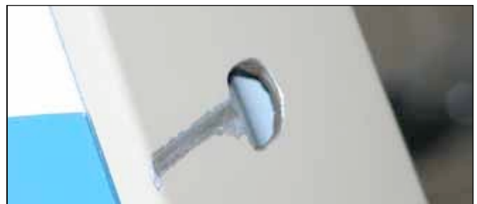
A simple striker plate of thin stainless is all that's needed to protect the airframe.
