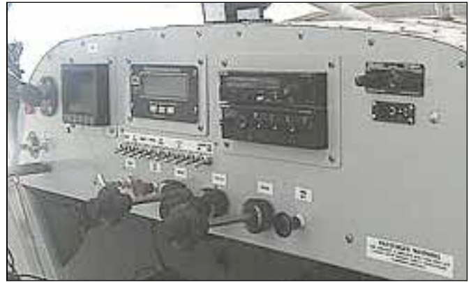
Electronics may not be traditional, but they sure yield a light panel. The Dynon display supplies all of the flight and engine parameters required.
