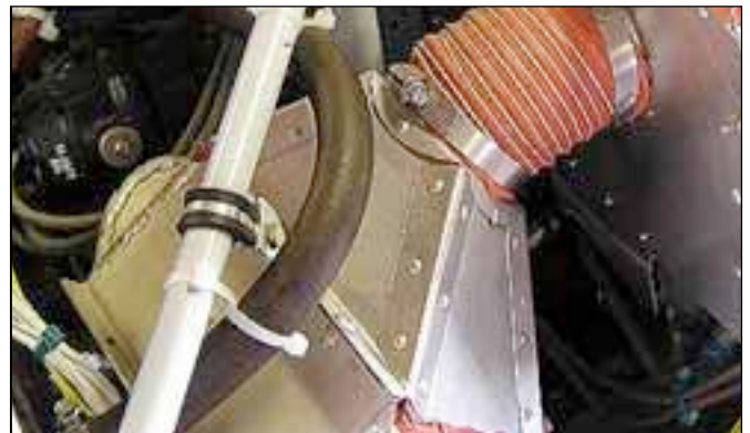
View from above: notice how deep the plenum is so the air can slow and transfer heat better. Inlet is 3" scat hose on the right, rear baffle. It's even better and simpler if the cooler is simply mounted right to the baffle.
