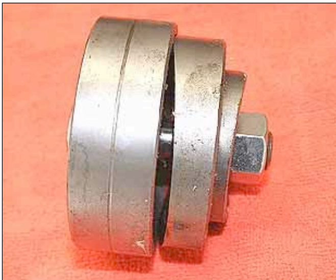
The Matco type of punch is more expensive but an absolute fool proof way of cutting a perfect instrument hole.
