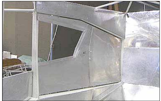
The builder has done a neat job of forming his upholstery backing panels. He can, if he wants, paint, rather than upholster them for a lighter interior.
