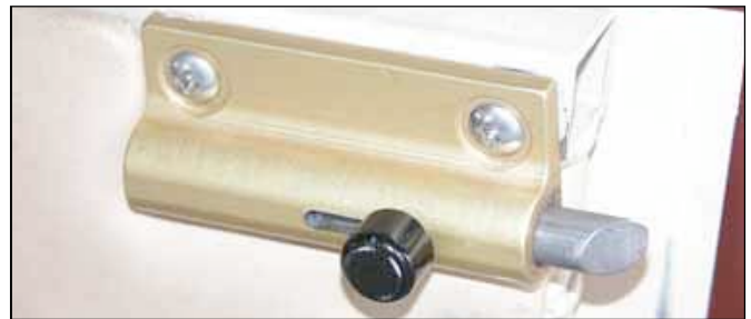
This is an alternate latch for the front doors that is available from Aircraft Spruce, PN05-04520/21. This latch lets you slam the door, rather than having to open the latch each time.
