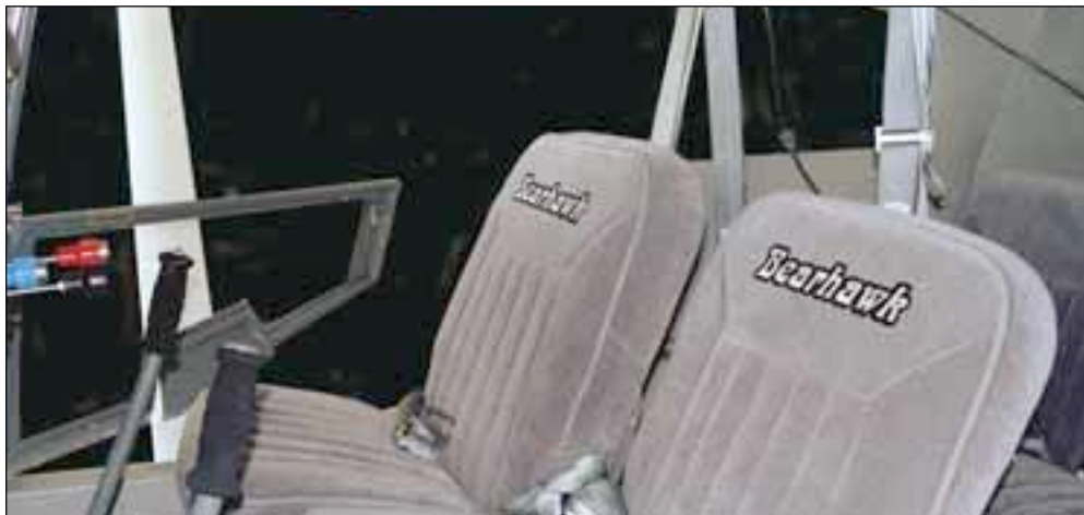
Pat Fagan's award winning BH uses Piper Cub technology in the interior: the sides and head liner are nothing but painted Stits PolyFiber. Light and durable. A variation could be to "flock" it as original Champs were done
