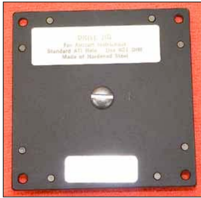
Inexpensive, hardened drill template locates the bolt holes before you cut the main hole.
