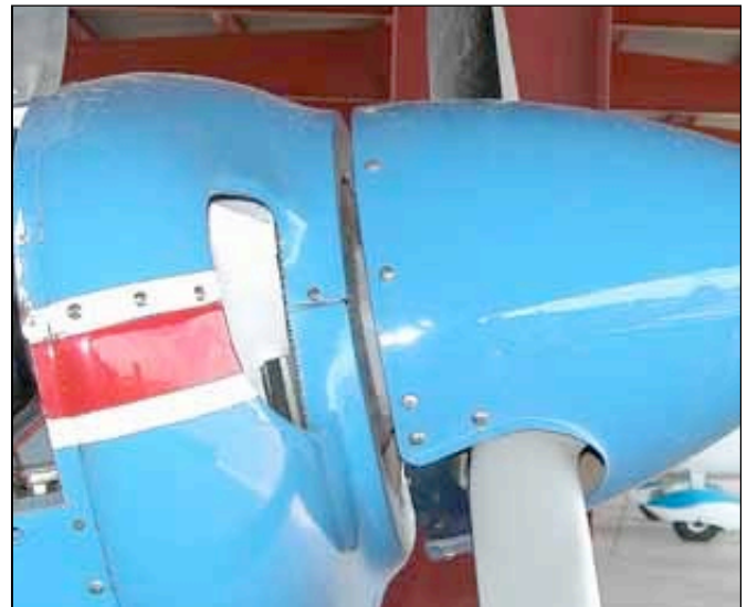
Jigging the nosebowl so it is square to the firewall horizontally and square to the crankshaft vertically, is critical. Don't make the nose gap less than about 1/4". 1.2" is shown
