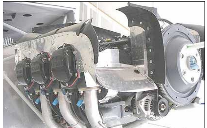
When trimming the baffles enough room must be left between the baffle and the cowling for the baffle seal.
