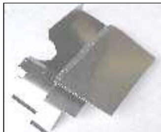
Van's Aircraft makes a complete baffle set for their RV-10 that is an excellent start for 540 Bearhawks.
