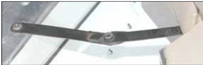
This over-center, hold-open device for the front door is found at local hardware stores and is another must have.
