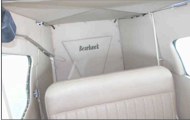
Leather is heavy, but soooo good looking. Notice how the headliner follows the “cathedral” shape of the tubing, which was meant to create more headroom in the back. If you go straight across from the longerons you give up about two inches of headroom.
