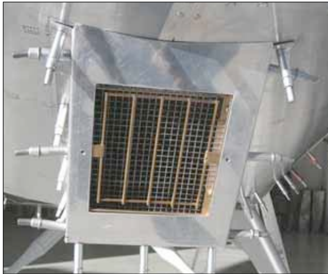
Front view of the completed air scoop, this on a 540 powered airplane. Notice the screen and bracket that is part of the Bracket Air Filter system that is attached to the front of the air box itself. Note the seam just above the scoop where the two halves of the bottom cowl are joined.
