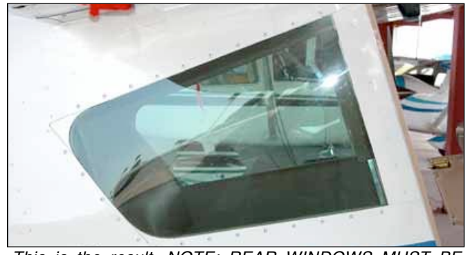
This is the result. NOTE: REAR WINDOWS MUST BE LEXAN AS THEY HAVE A BEND IN THEM. PLEXI WILL CRAZE IN TIME.
