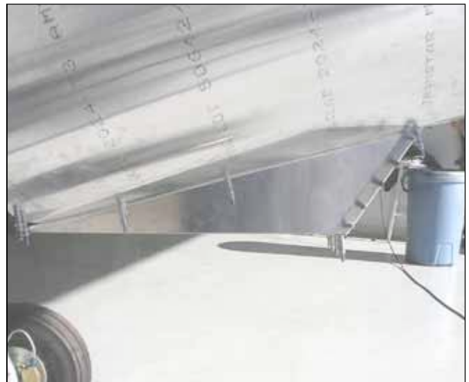
The scoop, as supplied will need only minor trimming before attaching to the bottom cowl, however every installation will be slightly different depending on engine and air box used.
