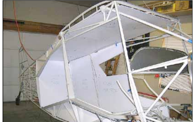
The interior shown with foam backing board trimmed to rough shape. Following the cathedral rear tubing is difficult with upholstery board but it's worth the effort.
