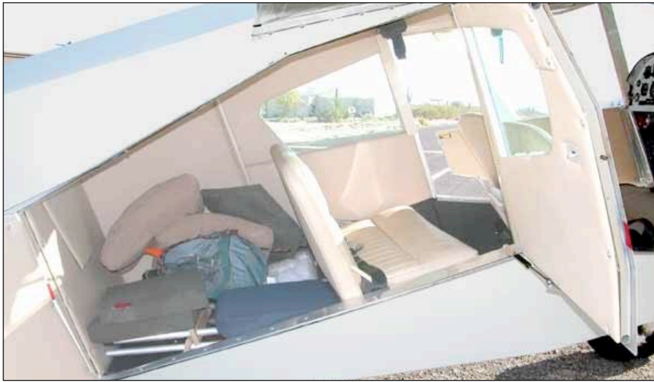
The doors, as they come in the kit, are complete and ready to install, but the builder must cover them with .025" aluminum, complete the latch assembly (or use a vendored latch) and install the windows.
