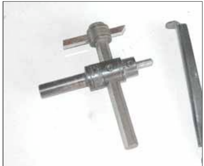
A fly-cutter allows flexibility in the size of the hole, but you have to be precise, when setting it up for instruments. Also, all work must be done in a drill press.
