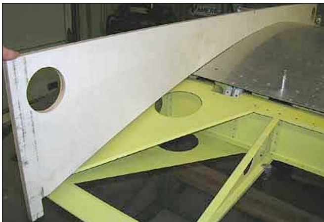
The supplied plywood template is the key to establishing the vertical placement of both the ailerons and the flaps.
