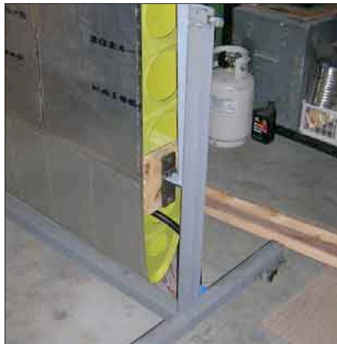
The construction uses 1" x 1/16 tubing as is used in security gates and can be found everywhere. Better yet, there's enough steel in the top of one of your crates to build the dolly.
