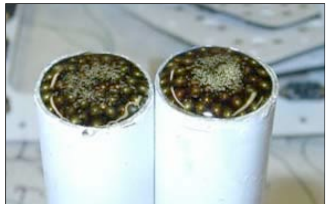
A plug formed of epoxy and shot keeps the loose shot in place.
