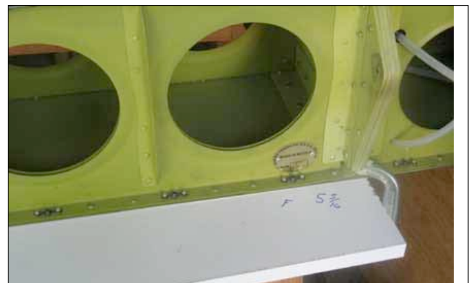
The plywood fastened to the bottom of the wing forms a datum from which to measure vertically to the edge of the bolt holes. We're looking for comparative measurements between the two wings. We don't care what the exact measurement is.
