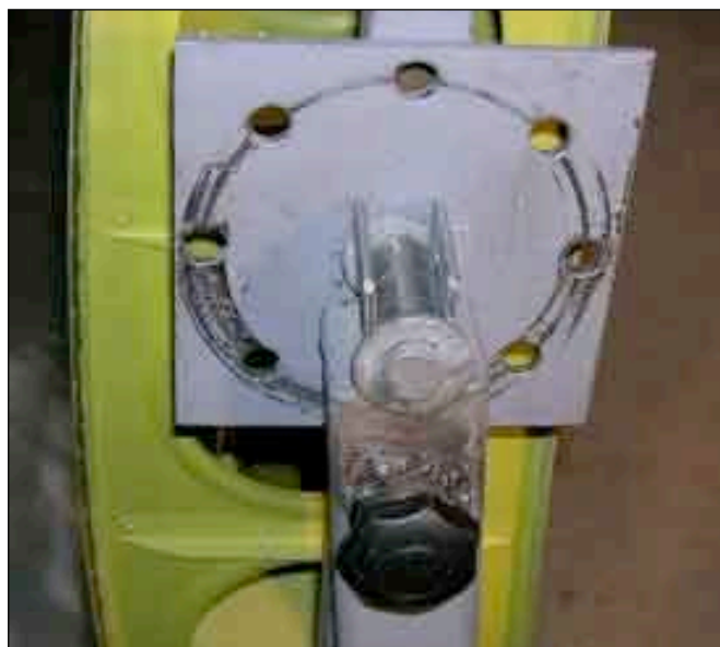
A locking mechanism doesn't get any simpler than this. The wing just lays in the pivot and the locking knob screws through a nut welded to the frame.
