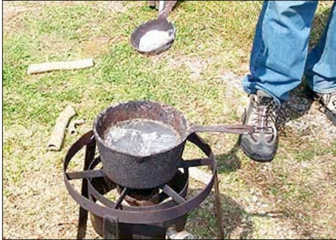
Lead can be melted a number of ways, but do it outdoors and avoid the fumes.
