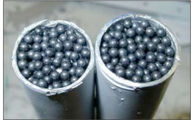
The smaller the bird shot, the fewer air pockets there will be. This is 8 1/2 shot and 12 would be much denser.
