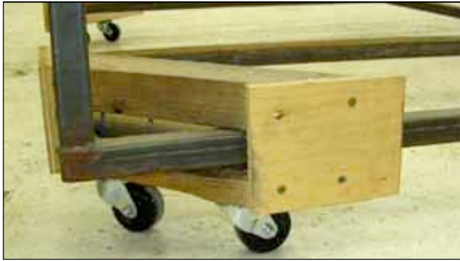
A set of easily made dollies for your wing crate makes them much easier to handle. An alternative are Harbor Freight furniture dollies.
