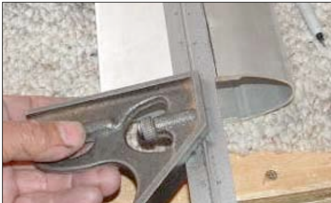
Mark a center line on both sides and both ends of the strut.
