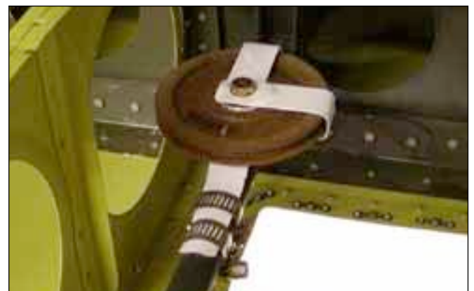
Front aileron pulley . Note the cable guard.
