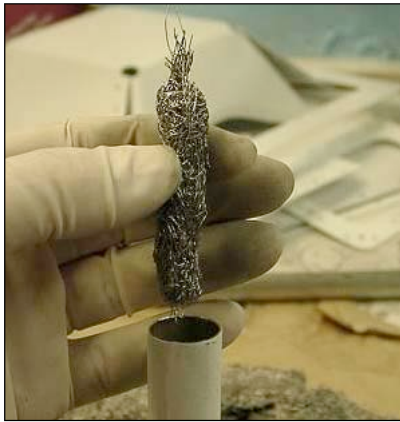
Lead wool "wienies" are formed really easily and tamped down are nearly solid.
