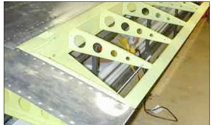
All of the control surfaces have tooling holes in the ribs that can be used for alignment: note the threaded rod holding this flap in alignment with the root ribs.
