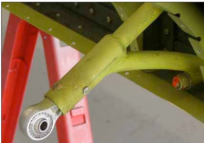
The control surface hinge bearings slide into tubes and are fixed in position by rivets or bolts. Prior to installation they can be adjusted in or out. After installation, their position can, to a lesser extent, be adjusted via washers under the hinge attach bolts shown
