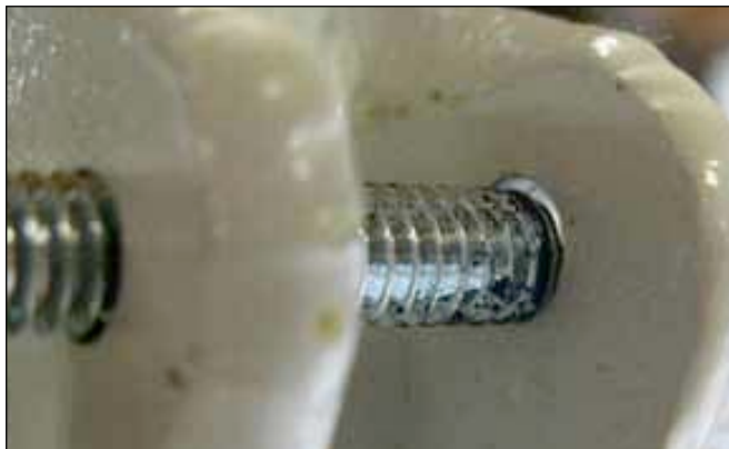
There will be a minor misalignment in the rear ear of the rear fuselage fitting, but this will be corrected in the drilling operation described in the text
