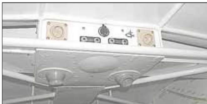
Jan Gutwein's superbly detailed rear vent system. He picks up the air in scoops on top the airplane.
