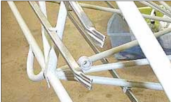
Whether aluminum or wood, the aft end of the stringers under the tail must be shaped so they move away from the fabric in a smooth fashion, with no abrupt or sharp corners.
