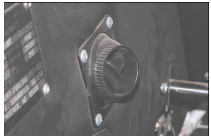
This is behind the NACA scoop above. Eyeball vents are available from all of the supply houses and offer a ready-made system to direct the air. Scat hose attaches to the back.
