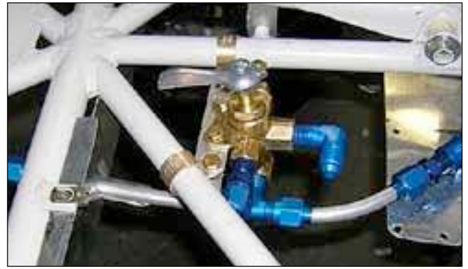
Another variation on mounting the fuel valve that will allow the builder to remove the floor boards with less trouble.
