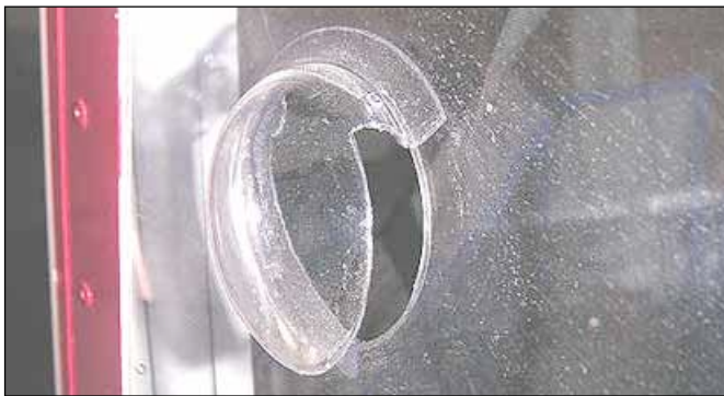
Simple and effective! It is installed in a side window and rotate forward, when you want a blast of air.
