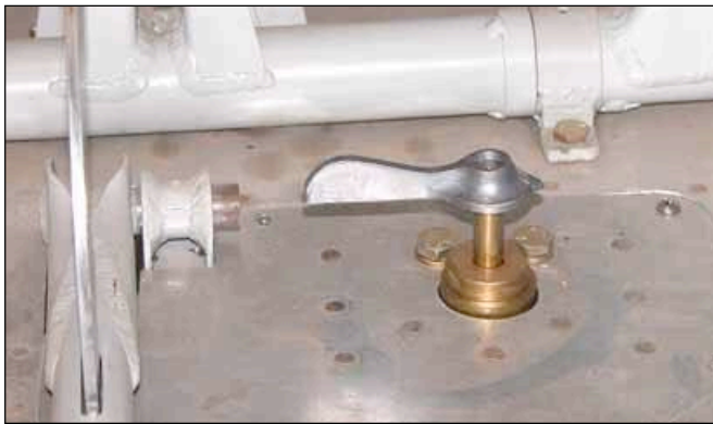
This builder mounted the fuel selector valve under his right thigh at the base of the flap handle for easier access. This requires a floor stiffening plate and a guard to keep from kicking it.
