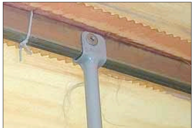
Almost anything can be used to fasten the stringer in the saddle including pop rivets, No. 6 bolts, etc.
