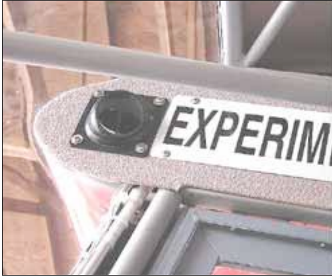
Cessna type wing root ducting can feed any kind of interior vent, in this case an eyeball vent
