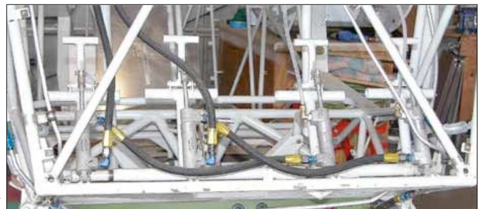
View from the front of a system using a firewall mounted reservoir and a parking brake.
