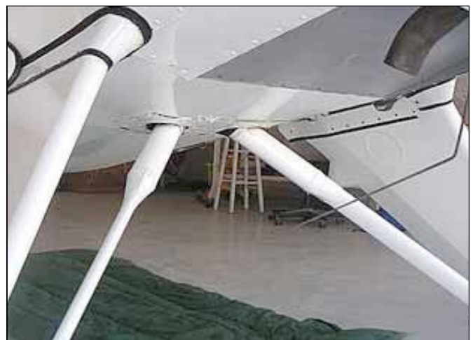
Normally the shock struts go through holes in the belly metal and room has to be left for them to move. This allows oil and exhaust access to the belly of the airplane. See following pictures for a builder's solution to that.
