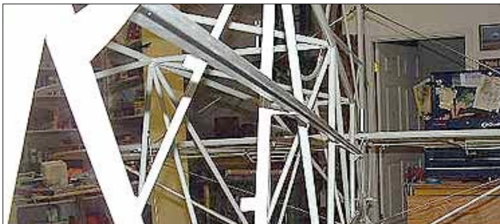
The stringers contribute zero strength but 100% of the shape. The better job you do of shaping and mounting the stringers the more smoothly the lines of your airplane will flow.
