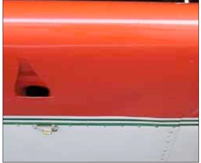
A NACA vent can be installed in the bottom of the wing. This what feeds the eyeball vent to the left. This vent CANNOT be installed in the .032 root section of the wing.
